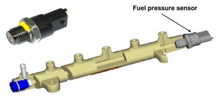
A fuel rail pressure sensor is located on the fuel rail.
