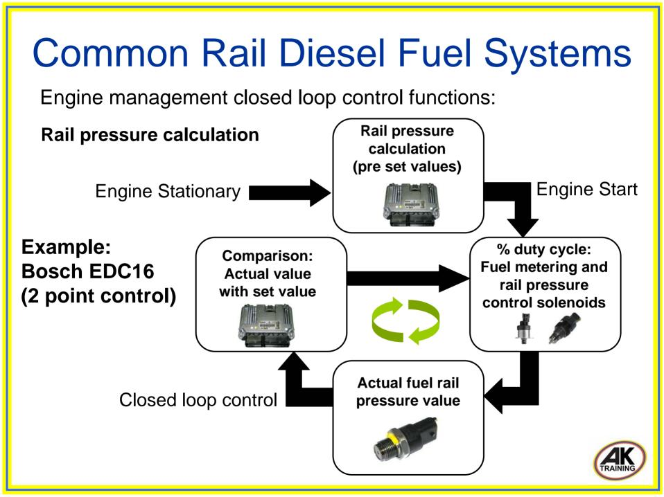
Engine management closed loop control functions:
