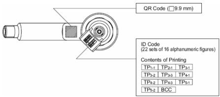
Bosch injector generation 2 IMA code for injector flow adjustment
