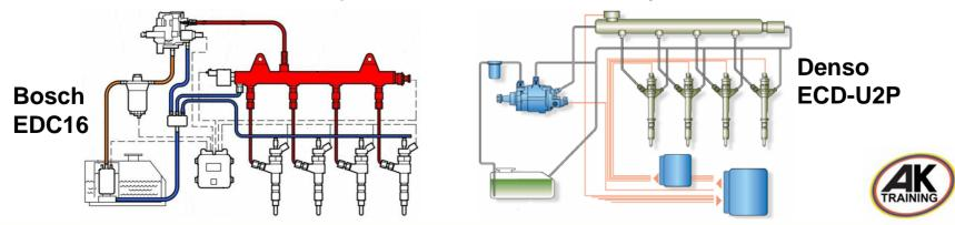
The fuel system can be divided into three basic circuits
