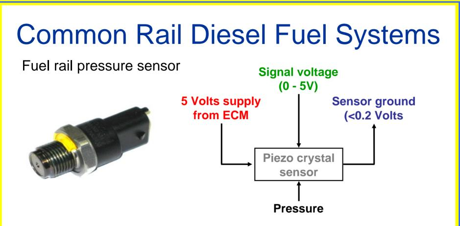
The engine ECM applies a stabilized 5 Volts supply to the signal wire of the fuel pressure sensor.....
