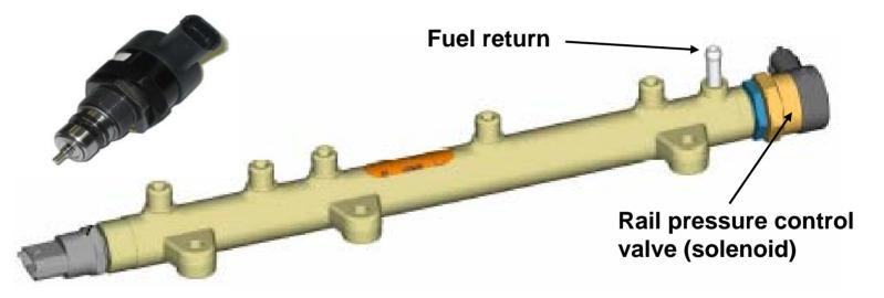
The valve controls fuel pressure by opening and closing a return port in the rail.
