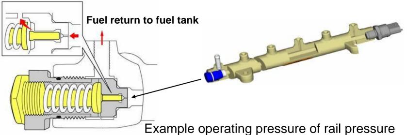
Example operating pressure of rail pressure limiter valve (Denso HP3 system):
