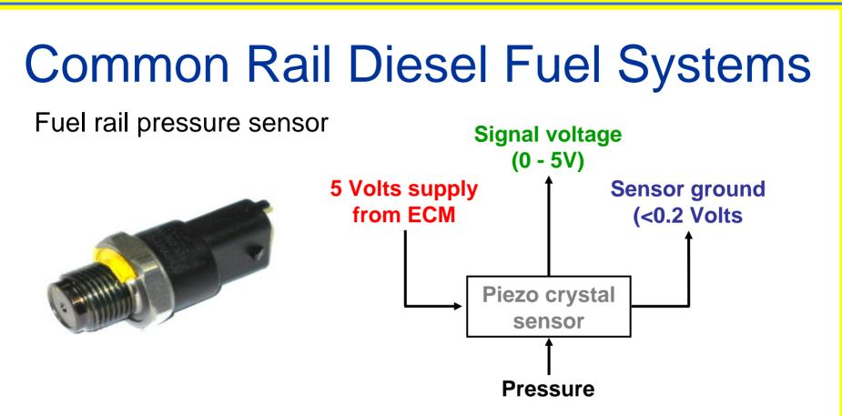
Typical signal voltages from rail pressure sensor:
